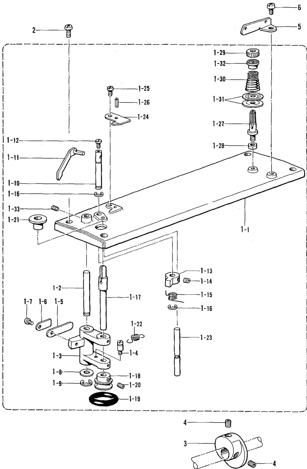
J. 糸巻関係/Bobbin winder mechanism/Spuler/
