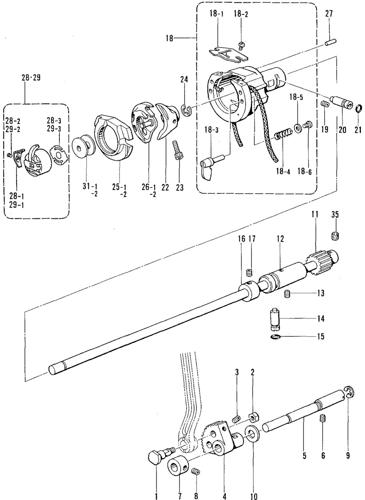
F. 下軸関係/Lower shaft mechanism/Untere Welle/
